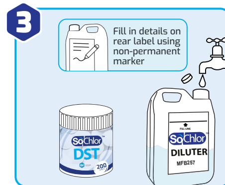
3 Dissolve the specified number of SoChlor tablets in cold water as indicated in the table below. Replace any solution older than 24 hours
